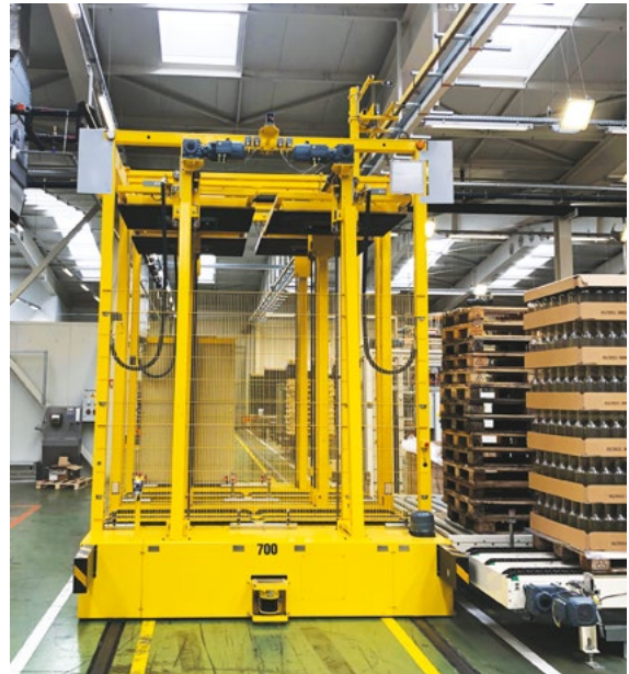
Mobile shuttle cars allow full and empty pallets to be transported without the need of a fork lift truck.
