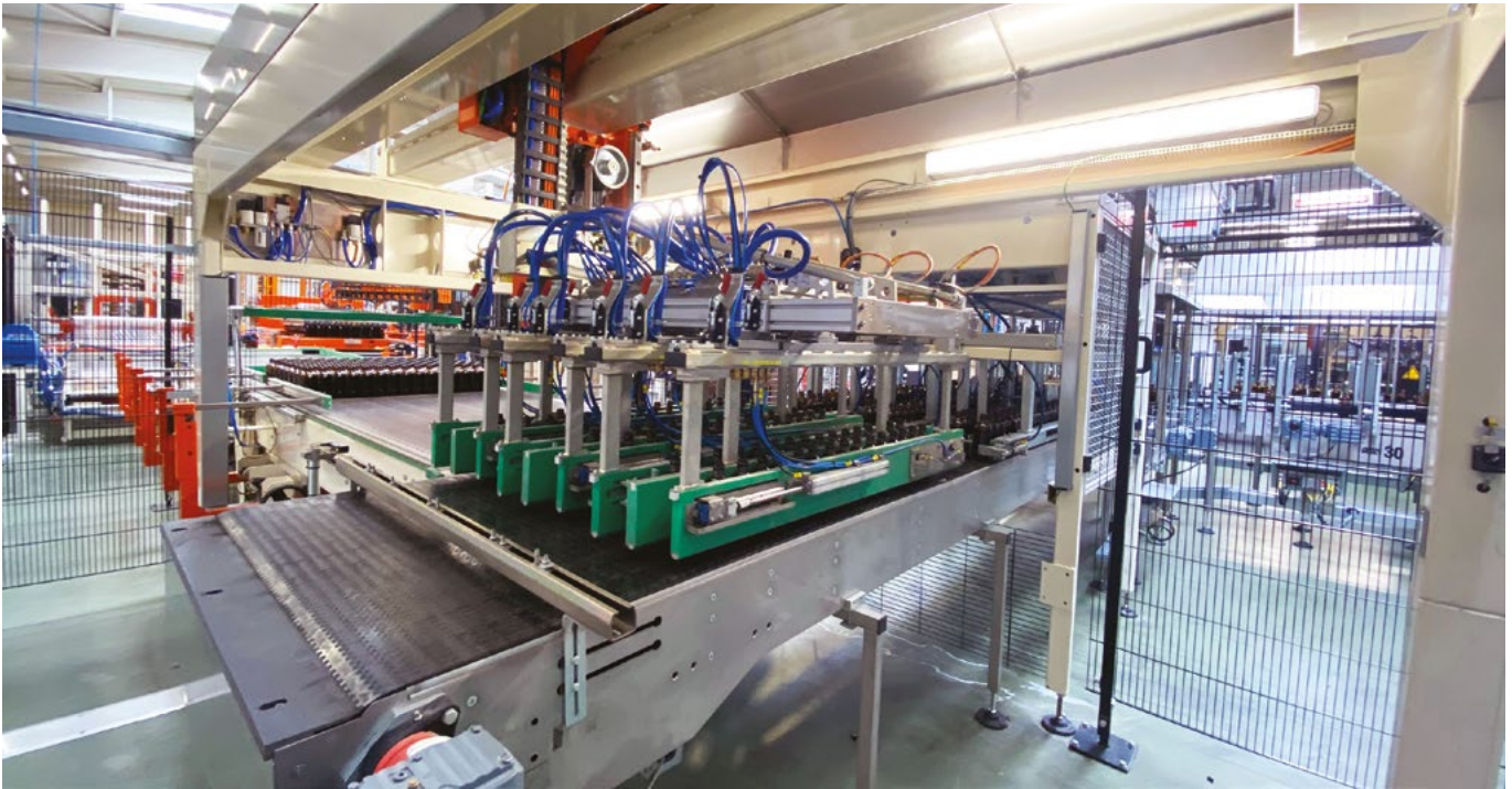
An open base frame maximises the stacker's accessibility.
