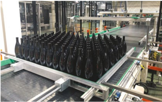
MSK layer formation for special bottle shapes.
